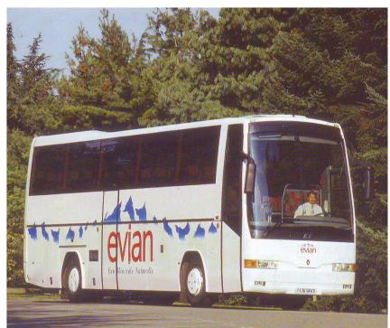
Customizing own bodywork, as specifications of RENAULT V.I., to exclusively sales in its network. Was adapted to the frame FR1 SX with a total height of 3.80 m, with the interior floor sloping and was designed, specifically for this release, a new front and rear with RENAULT lights. Two special units were built for the hospitality of the Formula 1 teams Williams and Renault Sport.
